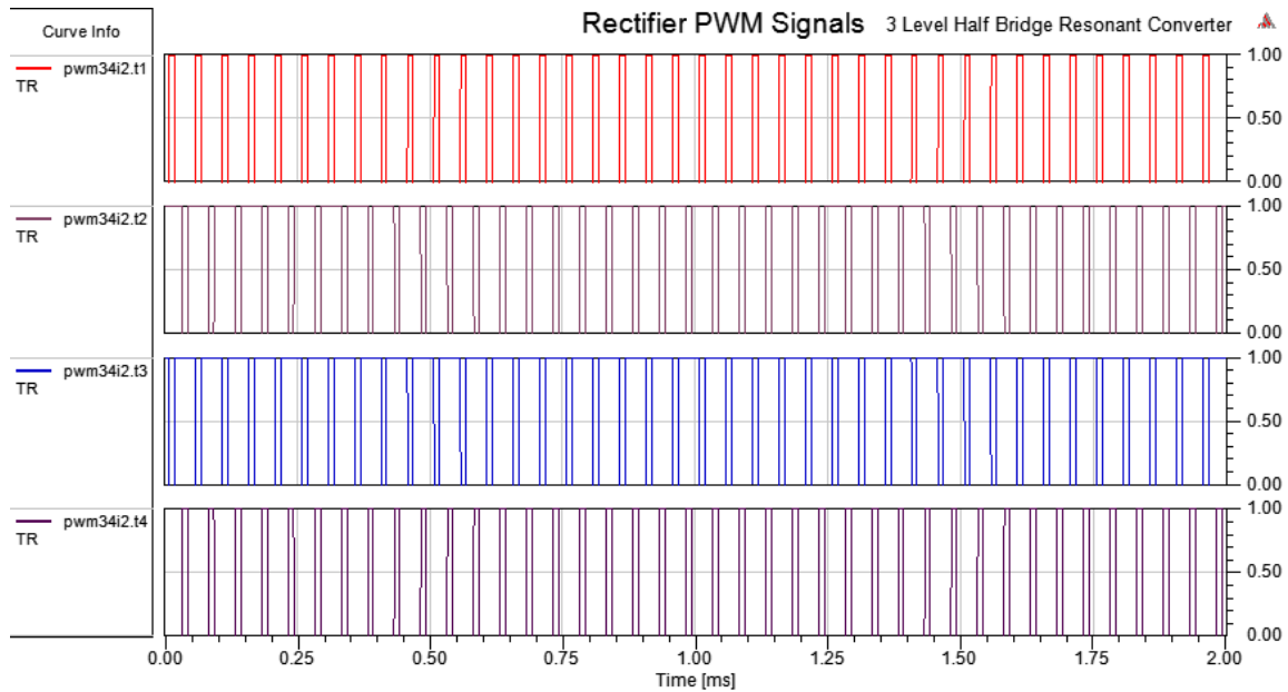
Figure 5: Rectifier PWM Signals
